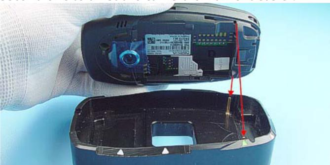
Place the unit into the Disassembly Jig SS-12. Note that guiding pins are positioned correctly into the gaps.
