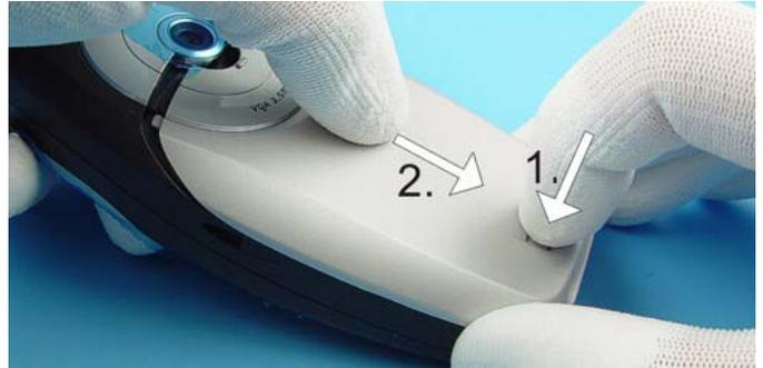
Press the Release Button before removing the C-Cover.
