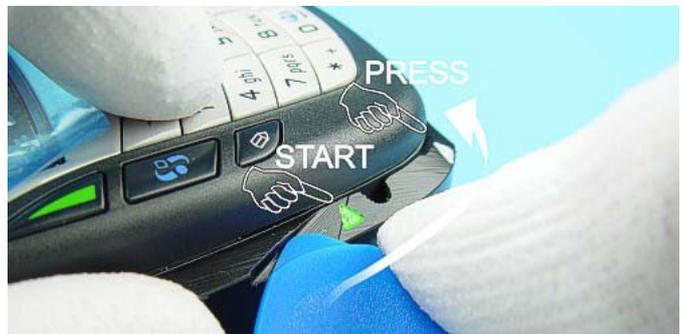
Place the SRT-6 on the Jig and shift it carefully along the edge of the Jig. Start at green mark to release the A-Cover, use it like a blade with moderate force only, to prevent damages at the covers. Shift the SRT-6 to the next mark and carefully press in the tip. (watch videos)
