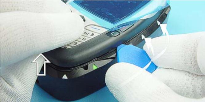
Lift the A-Cover on its bottom side carefully. Place the SRT-6 in the groove and shift it to the next mark. Then press in the tip as in the step above.
