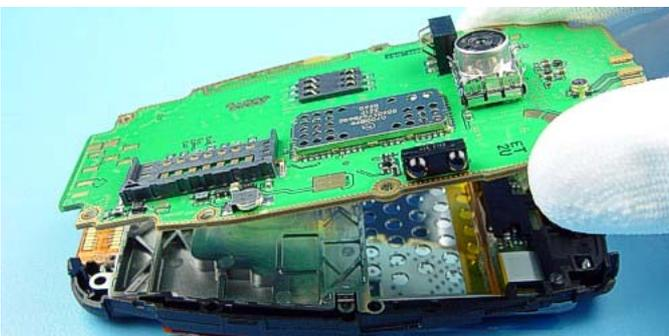
Now, the Engine Module can be removed.
