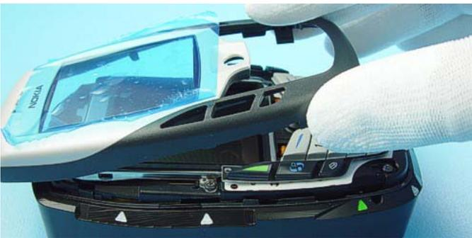
Now, the A-Cover can be pulled up. Always protect the inner side of the window and LCD with a film.
