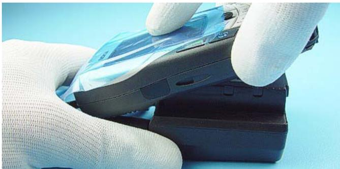
Insert the Flash Adapter SF-2 like a battery, start at the Battery Connector side.
